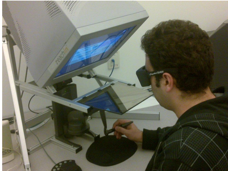
Figure 7.1. Haptic signature application. This figure shows a user signing his name on virtual background using a haptic device.
