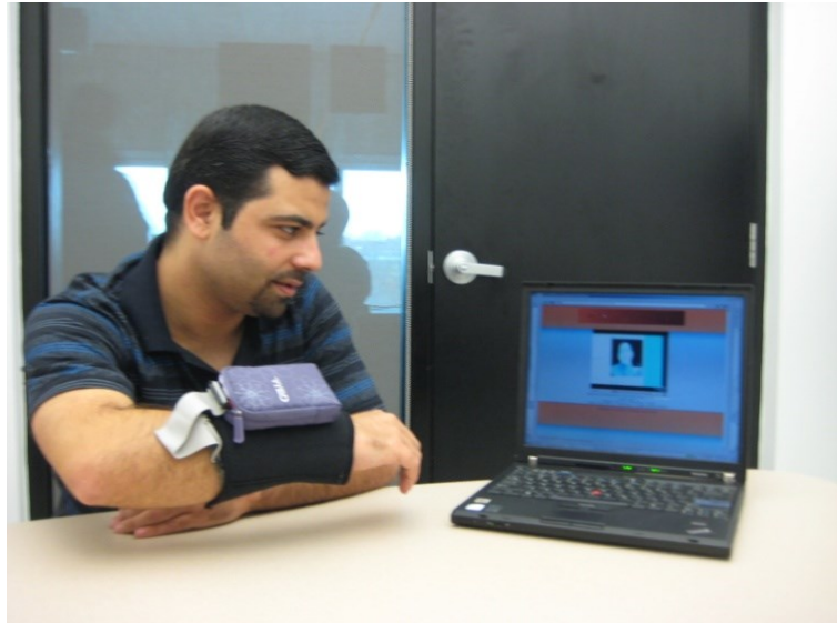
Figure 6.6. Experimental setup at the DISCOVER Lab. The user is watching a video and receiving synchronous tactile feedback via the arm bend device.
