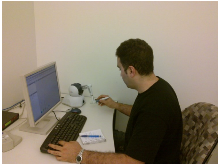
Figure 6.2. Experimental setup at the DISCOVER Lab. The user is manipulating the haptic device to write a particular letter on the writing pane.
